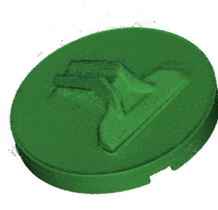
A scan made with Live3D before registration
